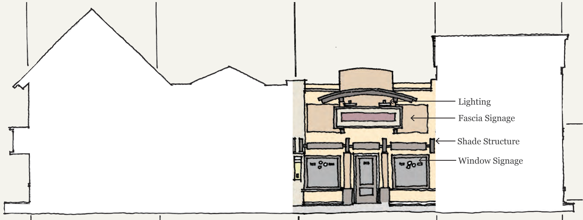
FIG. 10: TYPICAL BUILDING ELEVATION - LIGHTING
