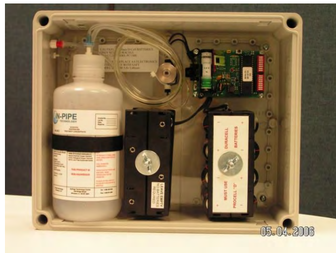
IPT Dosing Panel (Open)
