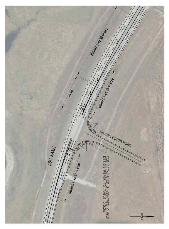
Figure 11. Proposed Intersection Improvement Concept Plan (South Access)
